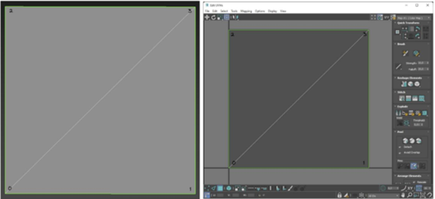
On the other hand, if there were a UV seam on the diagonal edge of this plane the situation would be different. **The vertices in the bottom left and top right corner of the plane now have two sets of UV coordinates so this plane will be split into a total of 6 vertices on import even though there might still only be 4 vertices in your 3d software.**
